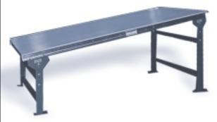
Inclined Outfeed Tables are constructed of a rigid sheet of UHMW polyethylene mounted on a metal frame equipped with adjustable legs. This allows the table to slope upward about 10" (254 mm) from front to back. As material exits the adhesive spreader, the leading edge travels up the table without disturbing the glue on the bottom of the piece.
