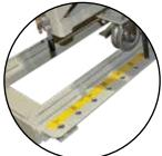
Added tape measure to conveyor to help operator more easily determine the conveyor position for various width boards.
