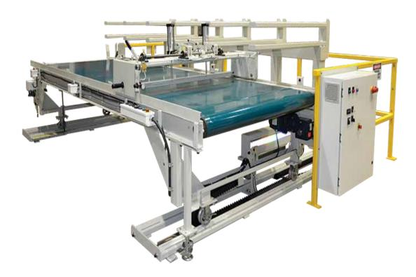
The Black Bros. Laminate Indexing Station (LIS) offers a convenient solution to what was once a difficult, messy task — handling heavy stock that is glued on both sides. The LIS eliminates the need to manually handle panels, leading to lower labor costs and increased production rates. The LIS positions the laminate in the same spot every time, so quality is consistent and laminations are cleaner.
