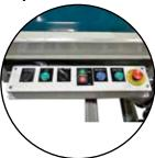
Added reset button to operators' side of conveyor for ease of resetting machine.
