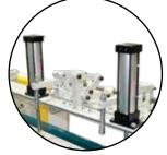
Air cylinders added to carriage to more accurately align lower substrate to the laminate.
