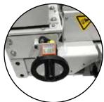
Added hand wheel with dial indicator for easier board width adjustment.
