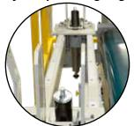
Air cylinders added to conveyor to more accurately align lower substrate to the laminate.
