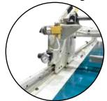
Changed carriage casters to linear bearing. This stabilized the carriage so it would better guide board to correct placement.
